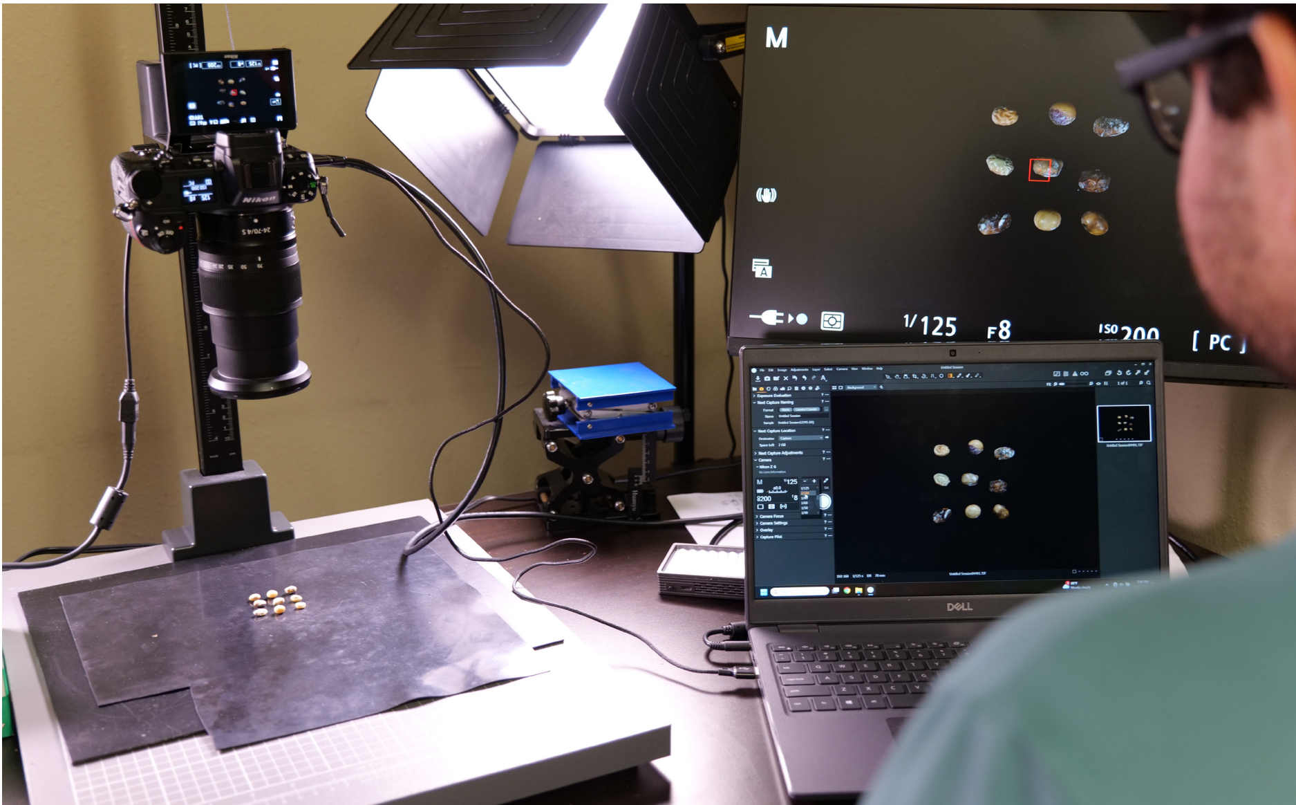
Soybean scanning and monitoring setup in Kevin Hoffseth's lab. Photo by Randy LaBauve
